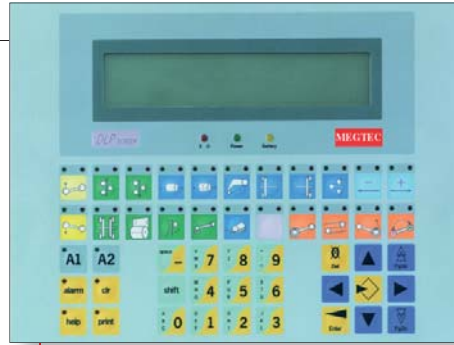
Operator control panel for paster setting with a display screen for status, fault finding, service diagnosis and help screens.
