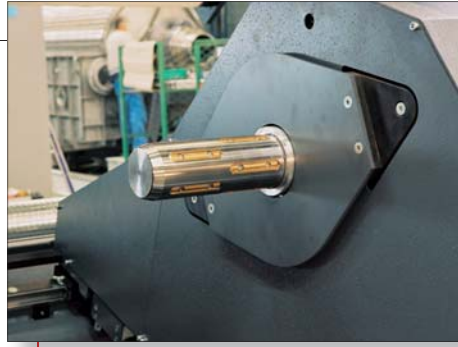
Standard quick changeover 76 mm and 150 mm (3" and 6") core chucks ensure flexibility and production safety.
