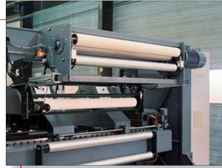
The splice arm was redesigned to minimize the distance between splice roller and splice knife to increase splice efficiency to over 99.5%
