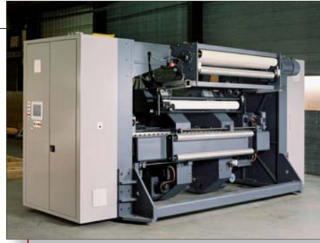
Key features include splicer turret with standard split arms, fully automatic quick changing chucks, 4 quadrant motors on each arm for drive and braking, pivoting splice arm and dancer assembly
