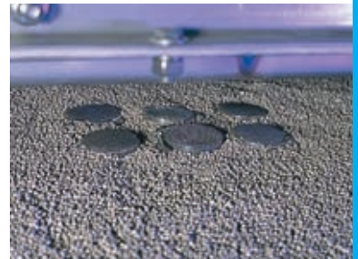
Catalyst testing is easy with pre-installed test cores. These provide a convenient cross-sectional evaluation of the catalyst bed for verifying performance.
